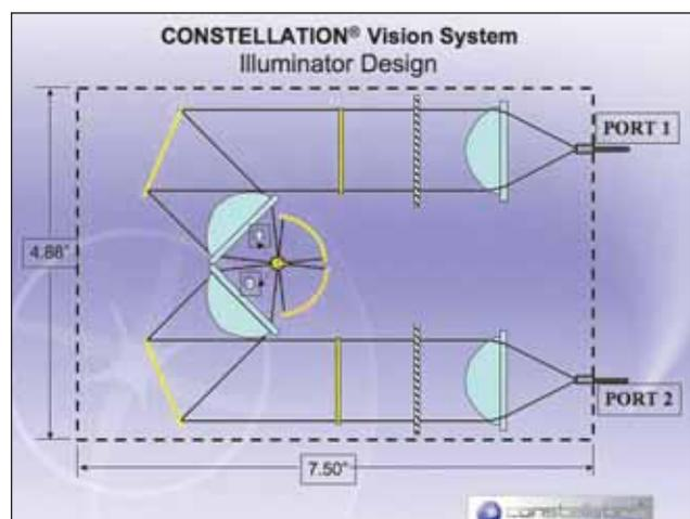
Figure 2. The illuminator design on the CONSTELLATION system.
