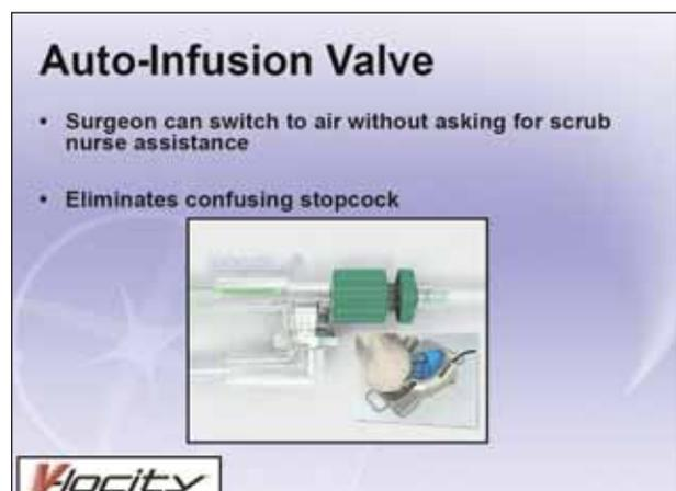
Figure 2. The auto-infusion valve allows the surgeon to easily switch to air without assistance from surgical staff.
